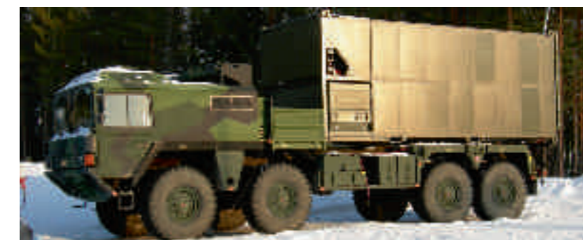
The mobile laboratories are housed in 20-foot containers and can easily be transported to the emergency scene by truck, boat or aircraft.
