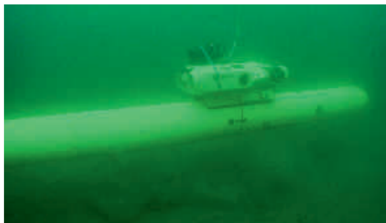
Sapphires can be launched from a submarine's torpedo tube. After a completed mission, a remote-controlled vessel grabs the AUV and guides it back into the torpedo tube.
