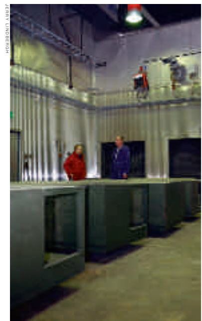
The climate hall offers temperatures between -52° and +63° and controlled humidity.
