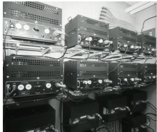
126. 5 W UK-station m/46, kraftaggregat
